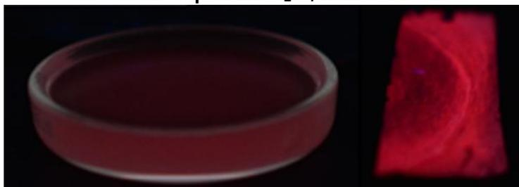
Chromium doped ZnGa<sub>2</sub>O<sub>4</sub> ablation solution (left) and deposited Nanostructures
